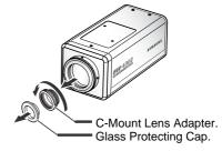
2. Attach the lens into the camera by turning clockwise.
